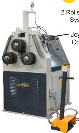
3R HPK-45 DRO option works for READ mode only. No limit feature available.
